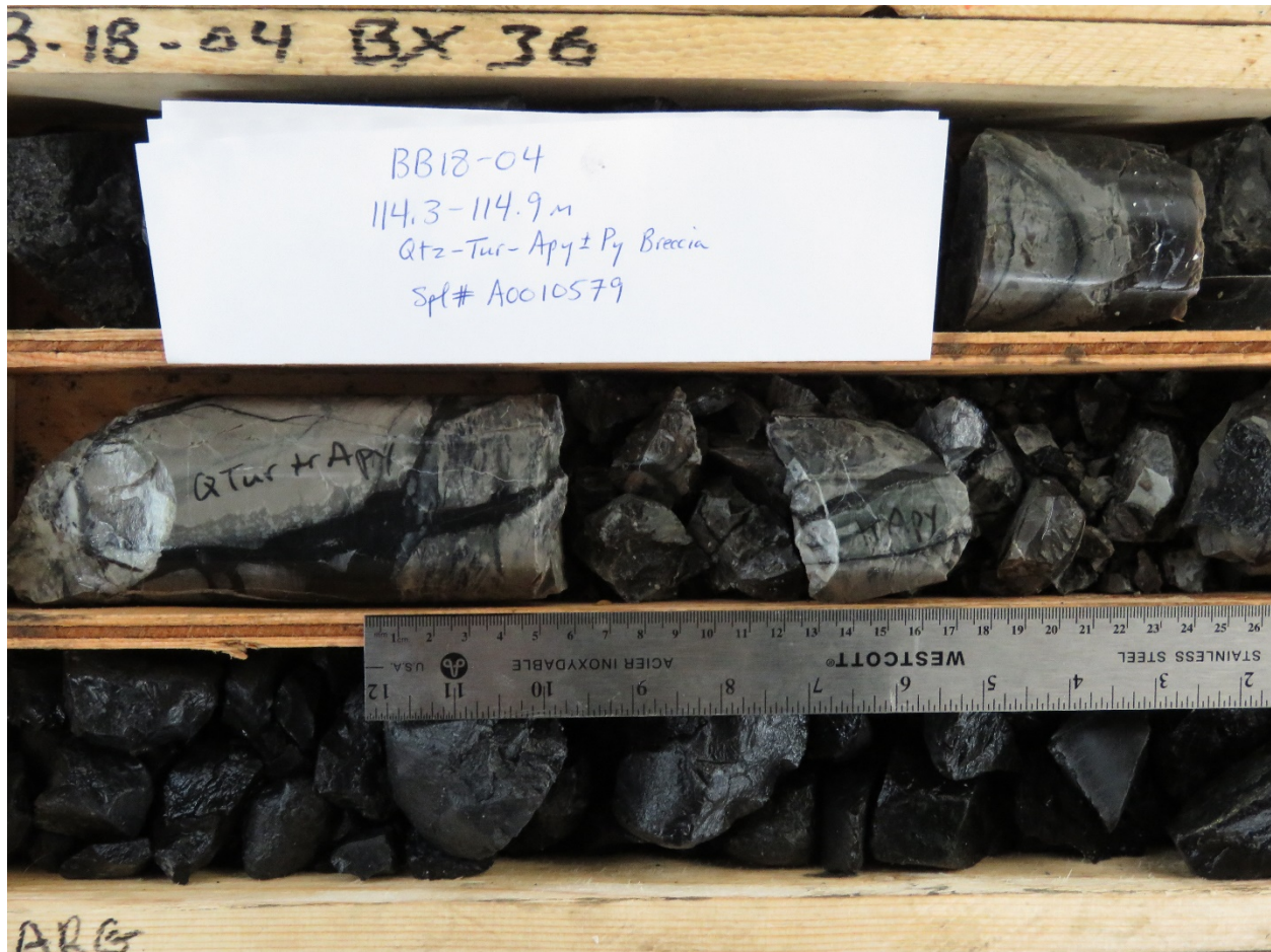
Figure 3 – Segments from 114.3 to 114.9 metres of drill cores from drill hole BB18-04 at Jaxon's Red Springs Project, which shows very strong silicified and sulphide quartz tourmaline mineralization
