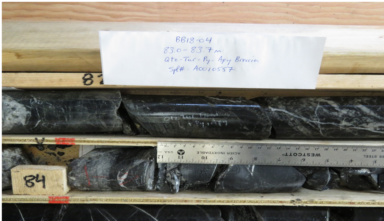
Figure 2 – Segments from 83.0 to 83.7 metres of drill cores from drill hole BB18-04 at Jaxon's Red Springs Project, which shows very strong silicified and sulphide quartz tourmaline mineralization
