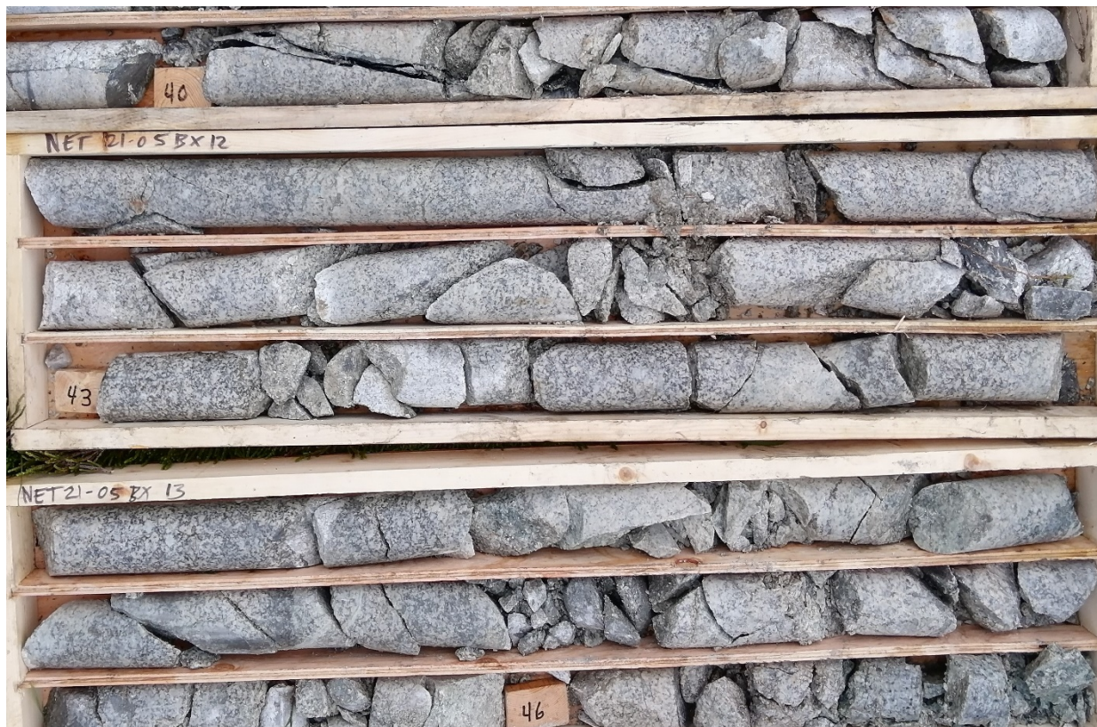
Figure 1. Cores from 40 m to 46 m from NET21-05 showing mineralized monzonite porphyry dykes.
