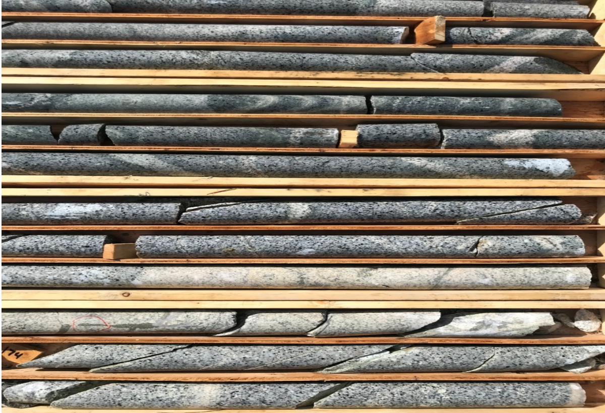
Figure 6. Core from 164.0 m to 176.0 m at hole NET21-04 showing multiple disseminated sulfides monzonite porphyry dykes.
