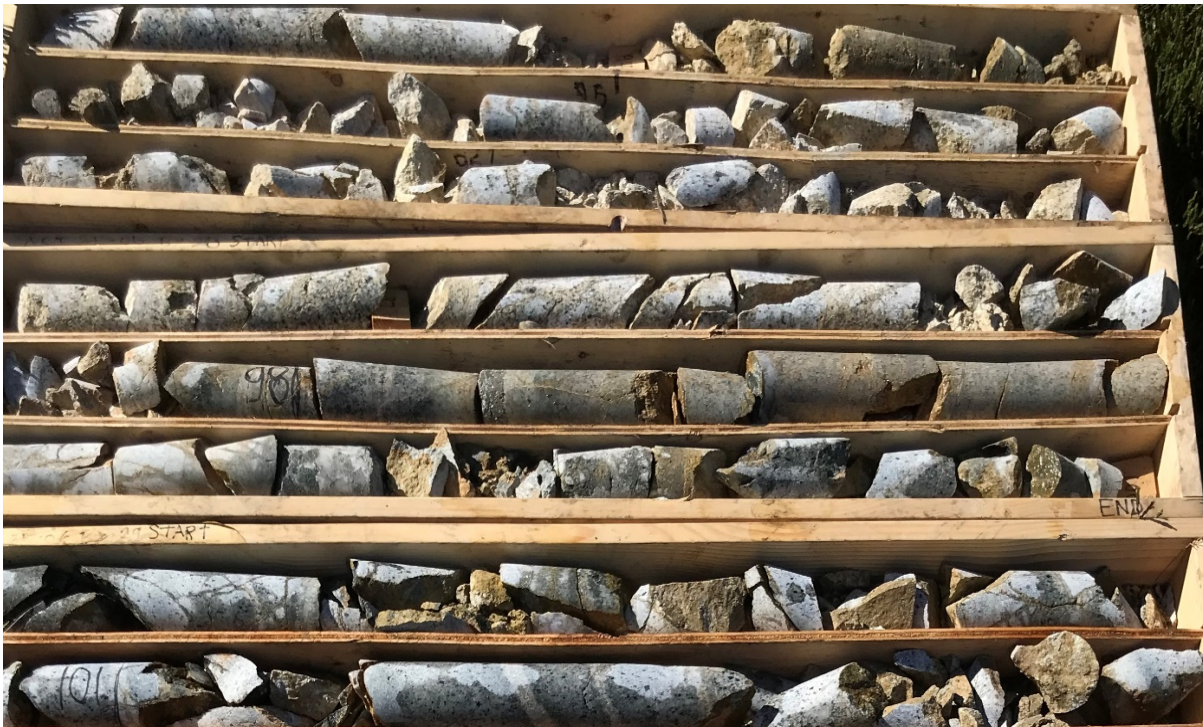
Figure 7. Core from 93.5 m to 100.5 m at NET21-06 showing multiple disseminated sulfide monzonite dykes; one large dyke from 98.0 m to 99.2 m showing strong disseminated and vein sulfides and silicification.
