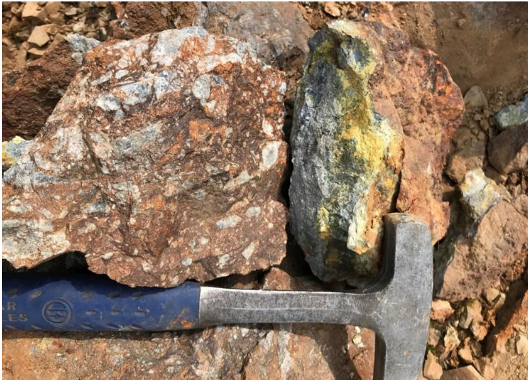
Figure 2. Grab sample 72030 assayed 923 g/t Ag, 2.68 g/t Au, 4.04% Sb, 8.39% Pb, 2.09% Zn and 0.36% Cu from the central part of the mineralization zone.
